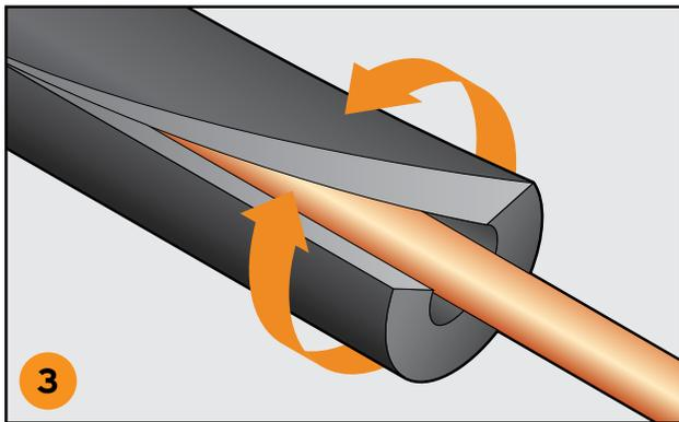
**4. Cutting:** use sharp non-serrated knives. Knife should be maintained at low angle to prevent tip from cutting/splitting inside wall. Cut flattest side of tube. Measure and cut all lengths (tube and sheet) long +1/8" [.32 cm] on each side (1/4", .64 cm) to install under compression. Use sharpened pipe cut-offs for holes. Glued seams should never be stretched and under stress.
