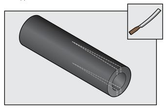
Glue notched edges together with AEROFLEX adhesive
