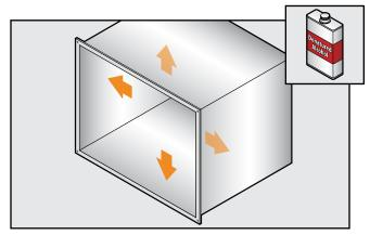
Measure duct dimensions and cut Breathe-EZ with PSA with straight edge.
