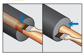
Glue longitudinal seams, butt joints and fittings with AEROFLEX adhesive. BEST PRACTICES/AEROFLEX ADHESIVES
