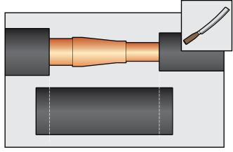
At one end, cut two equal notches out of opposite sides to fit smaller tube.
