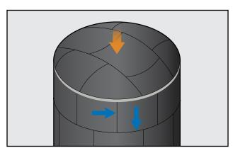
Once all sections of the dome are insulated, glue perimeter seam with Aeroseal adhesive under compression to create vapor seal.
