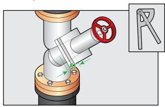
Transfer above measurements to AEROFLEX sheet and mark sheet accordingly.
