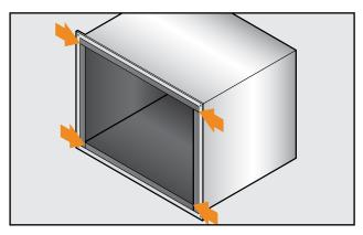
• Seal all transverse edges under compression with adhesive.
