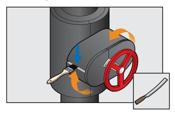
Glue edges of spindle housing jacket to valve cover body with AEROFLEX adhesive under compression.
