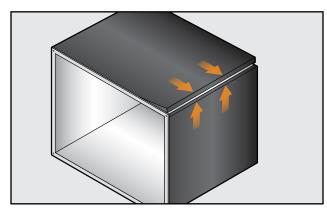
Apply adhesive to flush edge seams and allow to tack.
