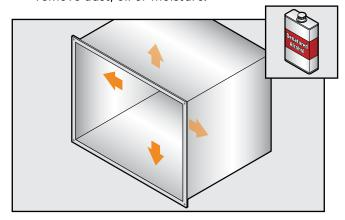
Measure duct dimensions and cut Breathe-EZ with straight edge.
