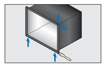
Glue four (4) flange cover edges to duct wrap with adhesive under compression to create vapor seal.
