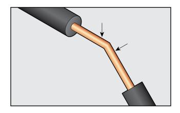
Cut AEROFLEX unslit tube at 22.5° angle using AEROFLEX Template and long sharp knife.
